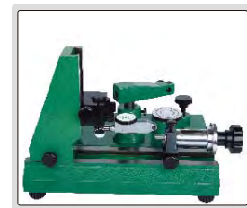
inspect accuracy of test indicators
