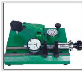
inspect accuracy of dial indicators (range 0-25mm)
