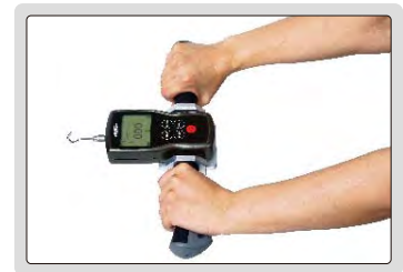
pull test with two handles
