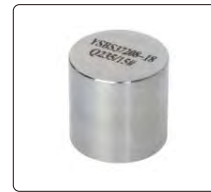
15# carbon steel control sample (optional)
