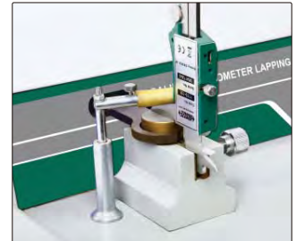
lapping measuring surfaces of caliper lower jaws
