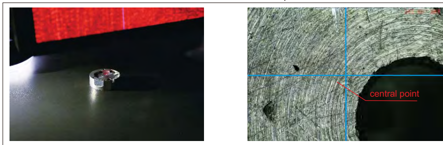
laser indicator locates the central point
