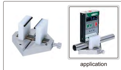
fixture for small shafts (optional)
